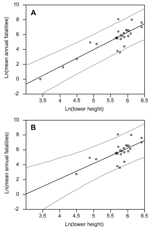
FIG. 1. Linear regression of  $\ln$ -transformed mean annual avian mortality by  $\ln$ -transformed tower height (m): (A) including all data points and (B) omitting two towers  $\leq 60$  m tall. Linear regression shown with 95% confidence intervals for individual values.
