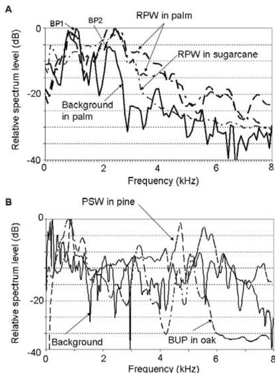
Fig. 2. Mean spectra of sounds recorded during a 1-min period from larval infestations: (A) RPW in palm trees (dashed line,  $n = 303$ ; dash-dot-dot line, 348 impulses) and in sugarcane (dash-dot line,  $n = 139$ ), and (B) BUP in oak branch (dash-dot line,  $n = 142$ ) and PSW in pine bolt (dashed line,  $n = 131$ ). Example spectrum of background noise is shown in (A) palm tree and (B) oak branch (solid lines), with background peak at 1 kHz marked as BP1, and peak at 2.4 kHz marked as BP2.
