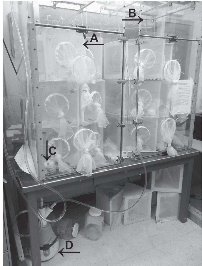
**Fig. 1.** Bug dorms. **A.** The large cage can house up to 12 bug dorms, with each stack containing 3 dorms. **B.** The large insect cage with humidifier attached. **C.** Stacks of Petri dishes. **D.** Humidifier.
