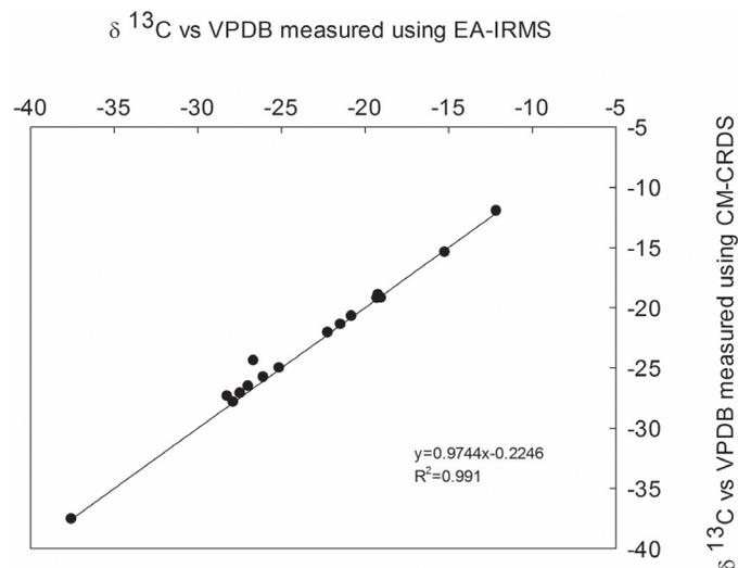
**Fig. 1.** Carbon isotope ratios of 16 different common dietary components measured using either elemental analysis isotope ratio mass spectrometry (EA-IRMS) or combustion module cavity ring down spectrometry (CM-CRDS).
