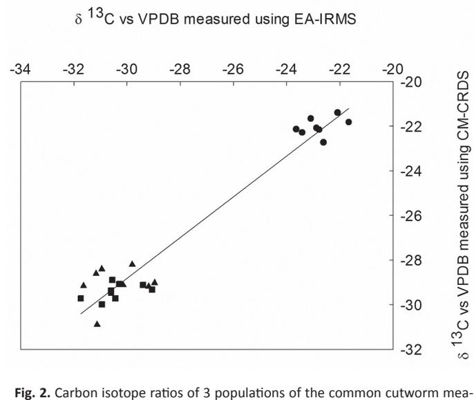
**Fig. 2.** Carbon isotope ratios of 3 populations of the common cutworm measured using either elemental analysis isotope ratio mass spectrometry (EA-IRMS) or combustion module cavity ring down spectrometry (CM-CRDS): Field-caught moths: squares; synthetic diet-reared moths: circles and laboratory-reared on castor diet moths: triangles.
