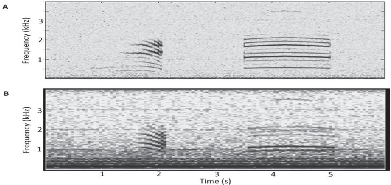
**Fig. 2.** Example spectrograms of a male call followed by buzzer response detected simultaneously by (A) accelerometer, and (B) contact microphone on the microcontroller platform. Darker color indicates greater energy at specified time and frequency.
