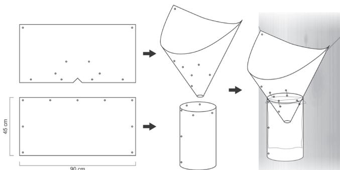
**Fig. 1.** Arboreal pitfall trap design. Two sheets of metal flashing are cut to length and punched with holes. Next, a cylinder and funnel are formed and secured with pop rivets or similar fastener. A plastic bag is inserted into the cylinder, and the cylinder and funnel are attached with tie straps. The bag is then filled with about 100 mL of 98% propylene glycol and secured to a tree trunk or branch such that arthropods slide down the funnel and into the collection fluid.
