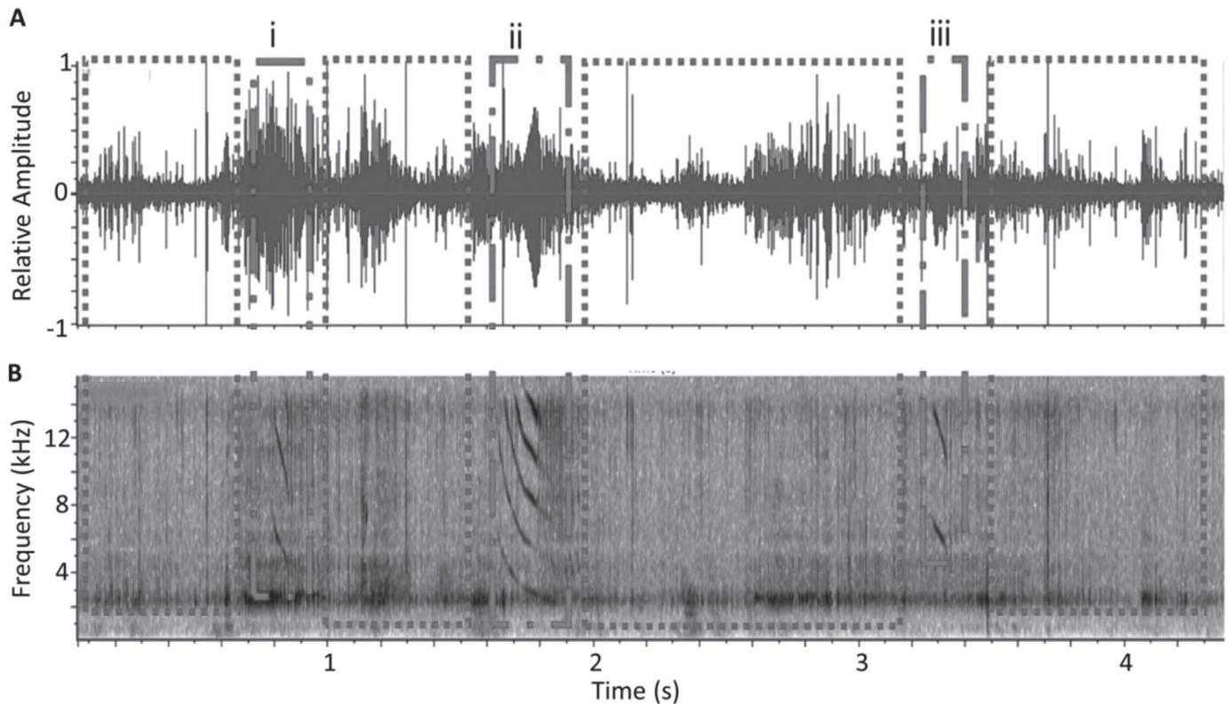
**Fig. 1.** (A) Oscillogram and (B) spectrogram of feeding sounds (dotted boxes) and squeals (dashed-dotted boxes labeled i, ii, and iii) produced by red palm weevil larvae in a date palm tree. In the spectrogram, darker color indicates greater energy at the specified frequency and time.
