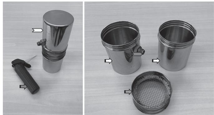
**Fig. 1.** The stainless-steel collection device was constructed to facilitate the collection of mites using carbon dioxide. Carbon dioxide cartridge with dust removing gun (dark arrow in left figure); carbon dioxide mite harvesting device (light elongated arrow in left figure); stainless steel canisters (light arrows in right figure); canister attachment device with wire mesh (dark arrow in right figure); entry port for carbon dioxide (dark elongated arrow in right figure).
