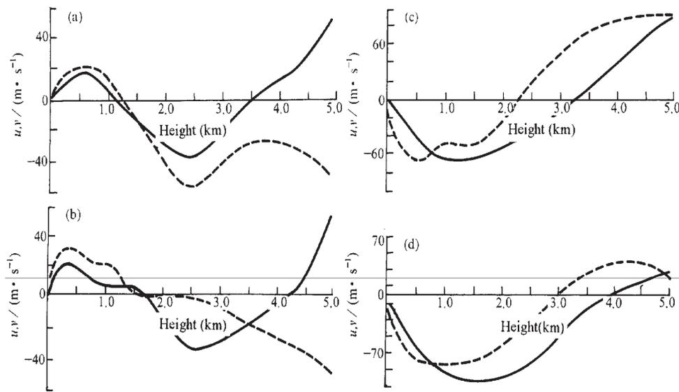
**FIGURE 4.** Vertical distribution of the composite wind field for 20 rainless days at (a) 2300 and (b) 1100 UTC, and for 33 rain days at (c) 2300 and (d) 1100 UTC at Chengdu. Solid and dashed lines are U and V components, respectively.
