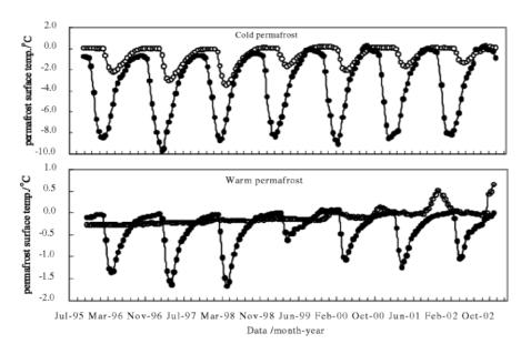
FIGURE 2. Permafrost temperature change at 6 m depth under the natural and engineered (asphalt) surfaces. Solid points are under natural surface and open points are under the central roadbed.
