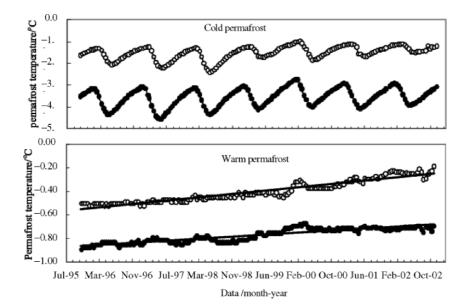
FIGURE 1. Permafrost surface temperature under the natural and engineered (asphalt) surfaces. Solid points are under natural surface and open points are under the central roadbed.
