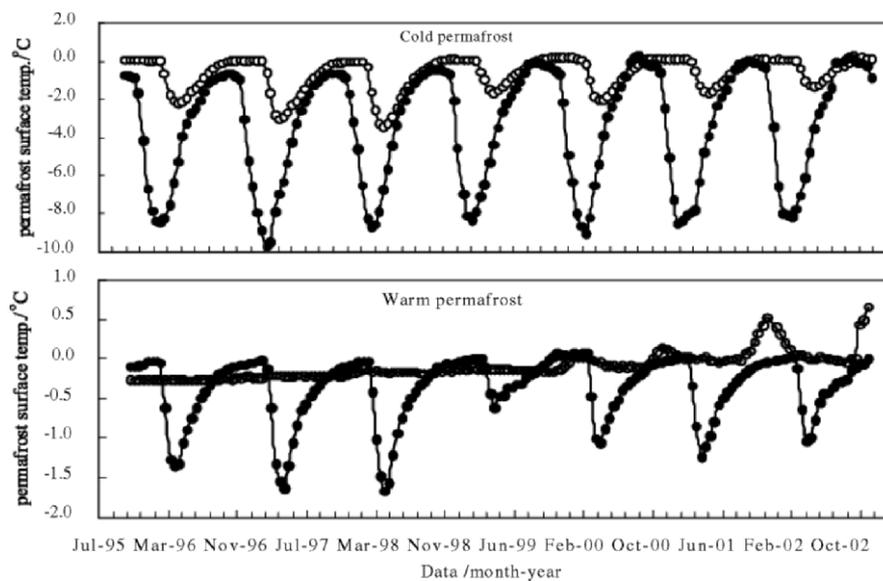
FIGURE 2. Permafrost temperature change at 6 m depth under the natural and engineered (asphalt) surfaces. Solid points are under natural surface and open points are under the central roadbed.
