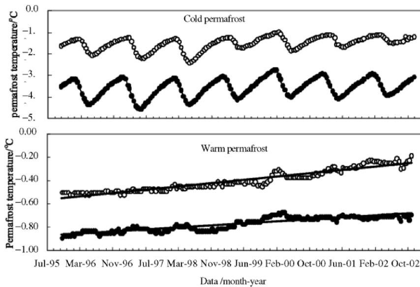
FIGURE 1. Permafrost surface temperature under the natural and engineered (asphalt) surfaces. Solid points are under natural surface and open points are under the central roadbed.
