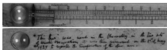
FIGURE 2. Newman (London) ivory spirit thermometer used on Franklin's second expedition (1825–1827). The lower half of the thermometer is shown with graduations in both Fahrenheit and Centigrade. The tube has been damaged. On the back of the thermometer is an inscription: “this thermometer was used in the observatory in the two sets of winter observations. It was then removed on the 1st May 1827 to register the temperature of the open air”. (On display in Scott Polar Research Institute Museum, Cambridge, U.K.)
