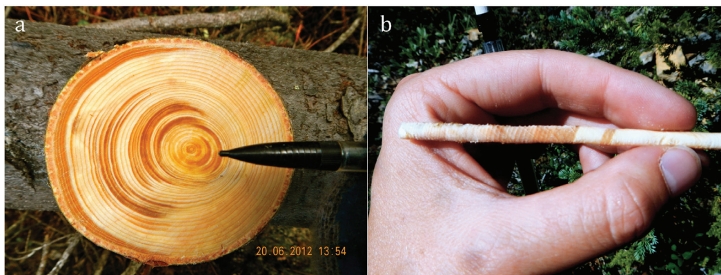
FIGURE 5. (a) Cross section (slice) of a 30-year-old spruce with reaction wood from about 20 years ago. The pencil shows the direction of avalanche flow. (b) Tree core showing growth rings and multiple sites of darker reaction wood. Many slices and cores were taken down the length of each path to track individual avalanche occurrences.
