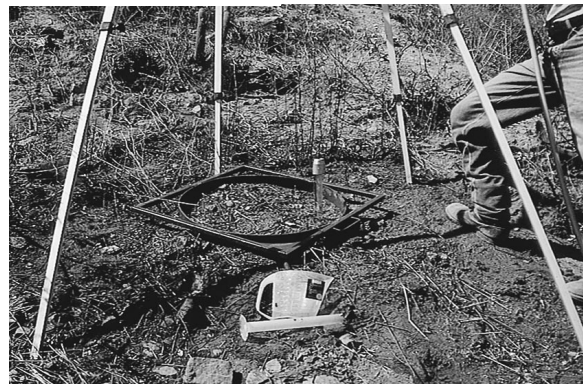
FIGURE 6 Rain simulation on an abandoned terrace in San Juan de Iris. (Photo by authors)
