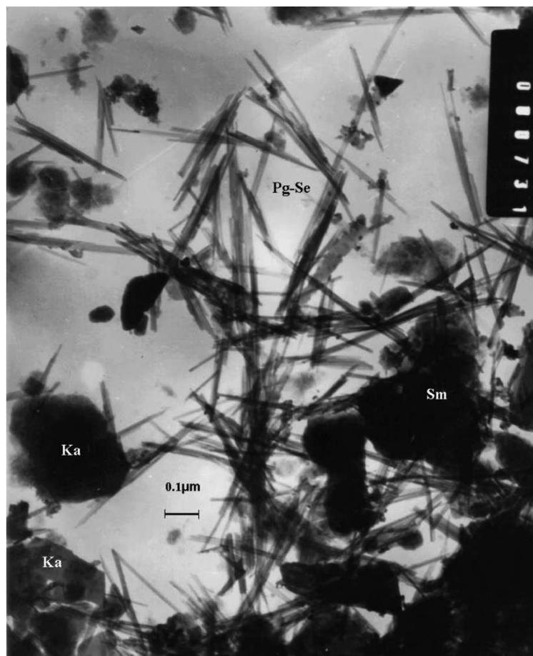
**FIGURE 3** Transmission electron micrograph (TEM) of palygorskite–sepiolite fibers in a sediment–clay assemblage with kaolinite, smectite, and other minerals in a sample taken at a depth of 7.5 m in the forested site. (TEM prepared by A. Adeli)
