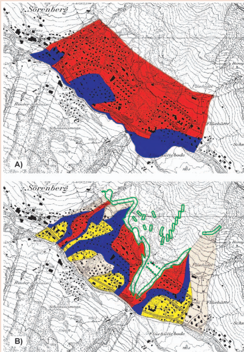
FIGURE 4, A AND B Hazard map for Sörenberg. Top (A) before, and bottom (B) after the implementation of the planned structural measures. Red: high degree of hazard; blue: moderate degree of hazard; yellow: low degree of hazard; yellow-white: hazards with a very low probability of occurrence; green: planned structural measures. (Maps reproduced by permission of swisstopo, BA035840)
