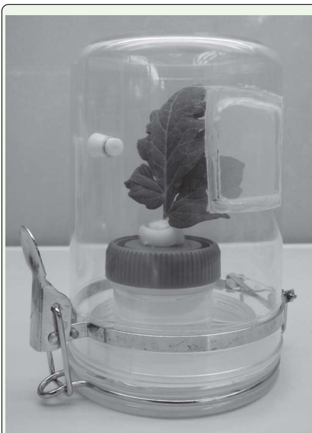
Figure 1. A clear plastic cell containing whitefly nymphs on a water-cultured tomato leaf used for the evaluation of host feeding and parasitism by whitefly parasitoids, Encarsia formosa .
