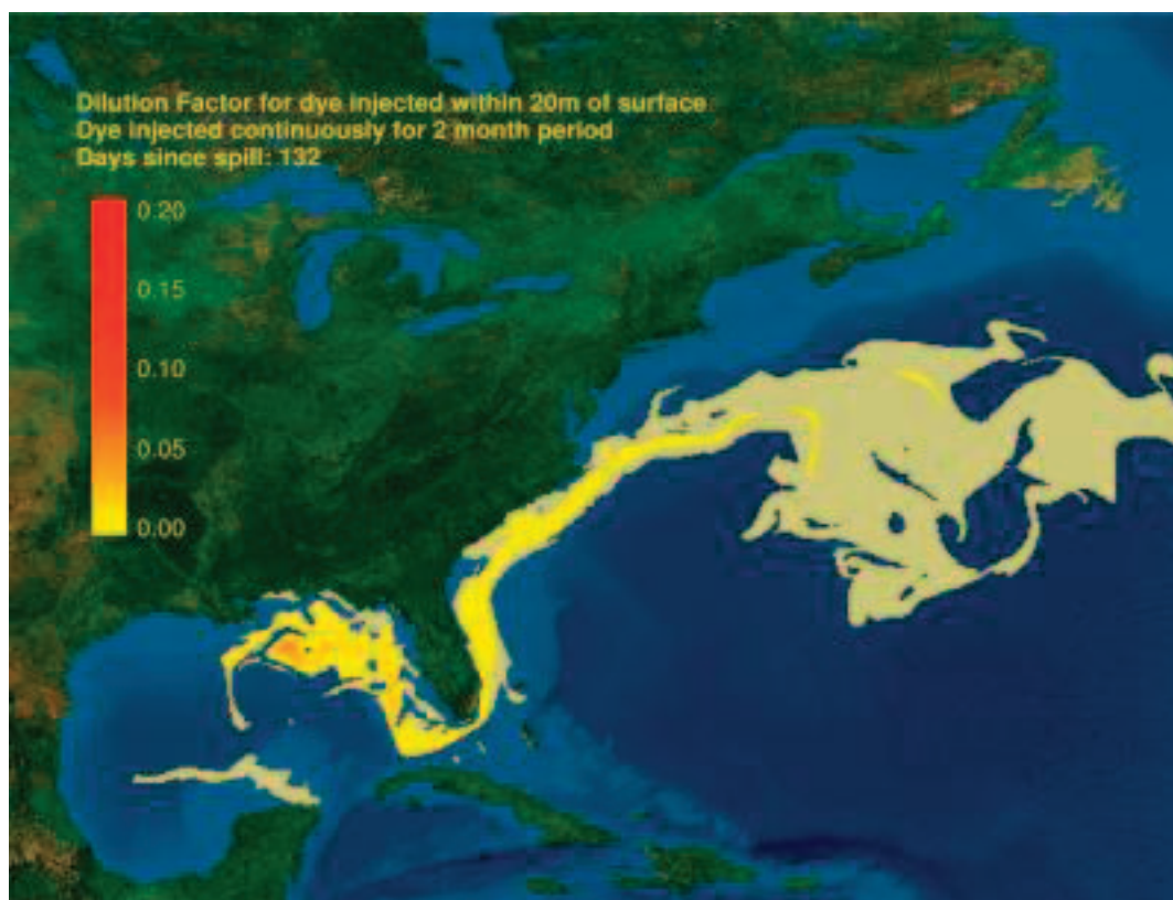
Figure 2. Oil trajectory after 130 days, predicted by the CCSM model for the Deepwater Horizon oil spill. Credits: National Center for Atmospheric Research and Department of Energy.
