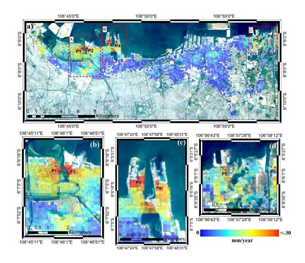
**Mean vertical deformation map in Jakarta coastal area.** The mean vertical deformation map above was generated using Sentinel-1 SAR data images between 2017-2020 using StaMPS algorithm. The mean vertical deformation map was overlaid with the depicted image from natural band combination (B4, B3, B2) of Landsat 8 OLI/TIRS C1 Level-1 taken on September 11, 2019, acquired by USGS.
