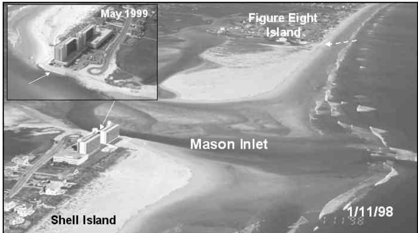
Figure 3. North view (1/11/98) of Mason Inlet and adjacent Figure Eight Island and Wrightsville Beach. Insert (5/99) shows oversize sand bags at base of threatened Shell Island Resort. Note clogged interior channels and position of ebb channel.
