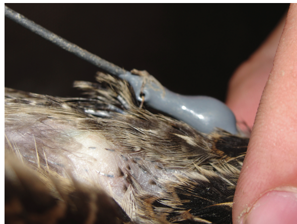
Figure 3. Radio-transmitter suture attachment to a ring-necked pheasant chick during summer 2010, Kiowa County, KS, USA.
