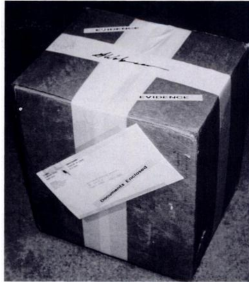
FIGURE 5. Method of packaging specimens for shipment to another laboratory. Labelled specimens are placed within a container that is sealed with tape, signed and clearly marked "Evidence." The covering letter and request for analysis are sealed in an envelope, labelled "Documents," that is attached to the outside of the container. The entire package, as shown, is ready to be wrapped in a separate outer wrapping that will be addressed to the laboratory.
