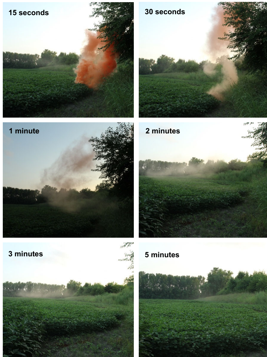
Figure 3. A time-lapse series following the release of a smoke bomb at a soybean field adjacent to a pipe river. The river is on the other side of the distal tree line. The visible plume first moved vertically. As the plume reached the height of the tree line, between 30 s and 1 min, it began sinking, which is likely the result of being incorporated into a cooler air stream. The particulate did not disperse but moved as a dust cloud to the low point in the field, where it remained visible for 3 min. (These particular smoke bombs, Enola Gaye smoke grenades, are designed to emit an observable plume for 90 s.)
