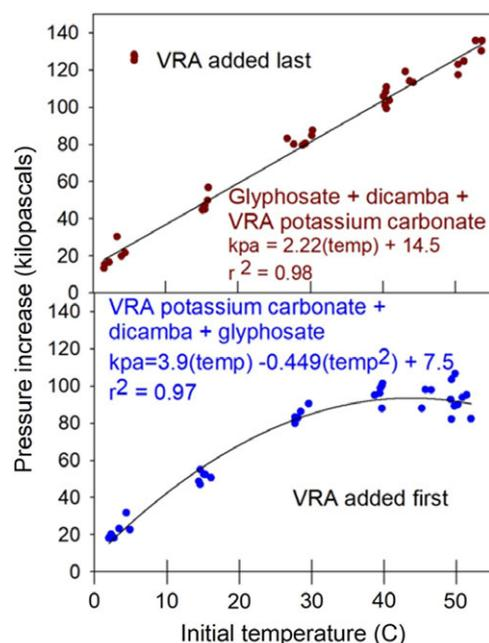
**Figure 2.** Effect of water temperature on resultant pressure increase related to the addition of potassium carbonate into the spray mixture last (top) or initially into the spray mixture (bottom). Data points represent individual observations at the respective temperatures. Regression equation details in text.
