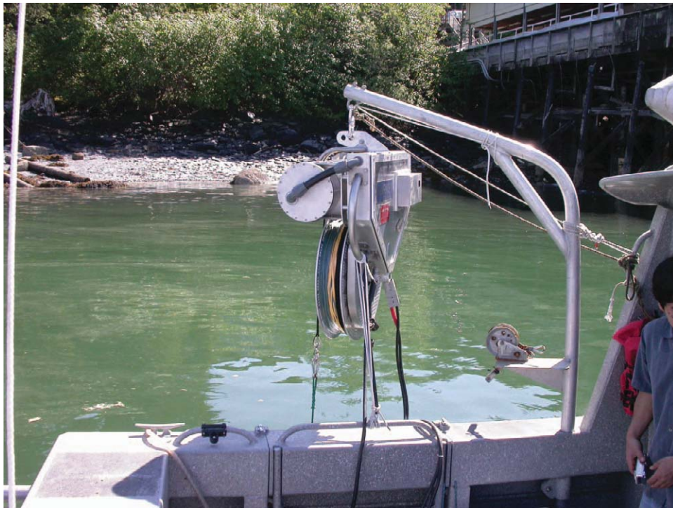
FIGURE 3. The Sidewinder block winch suspended from the davit of the 7-m RV Quest .
