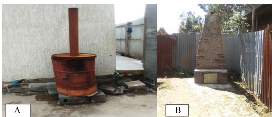
Figure 4. Sample photos of (A) unacceptable incinerator and (B) acceptable incinerator used to treat dry and infectious wastes.
