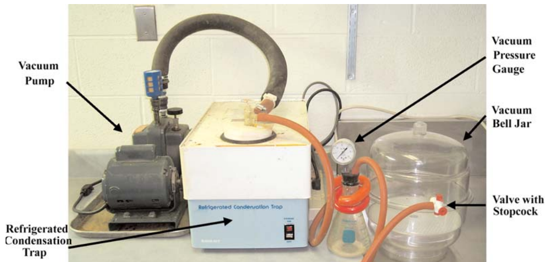
Figure 13. The vacuum-infiltration apparatus. The vacuum pump, refrigerated condensation trap, vacuum pressure gauge, bell jar, and valve with stopcock are indicated by arrows.
