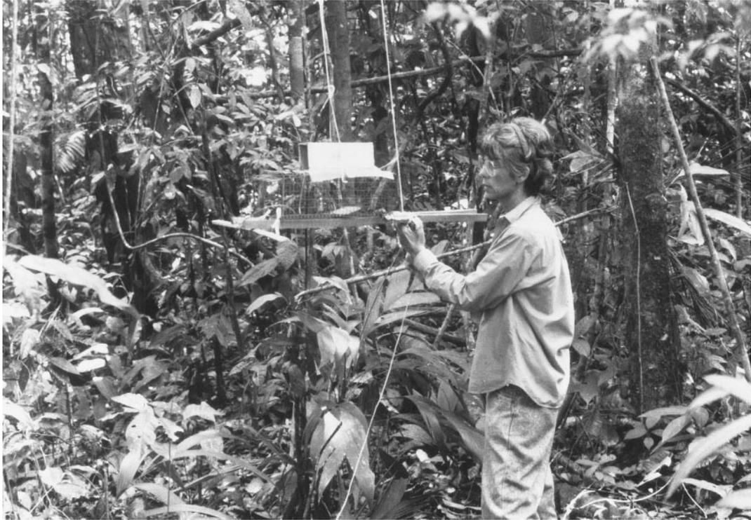
Fig. 14. A Malcolm-style (Malcolm, 1992) canopy platform operated by a pulley and line system and carrying a Sherman live trap placed on top of a Tomahawk live trap. Photograph taken by M. N. F. da Silva in September 1991 at Seringal Condor (locality 6).
