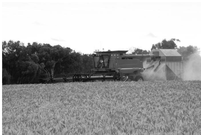
Figure 1. Chaff cart system in operation during commercial wheat crop harvest.
