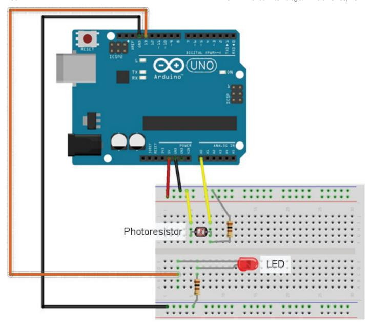
**Fig. 1.** The schematics for 4 laser trip wire systems on a single breadboard and a single Arduino board. Lasers have been excluded. Note how the Arduino board allows for the hybrid use of both analog and digital circuitry systems.
