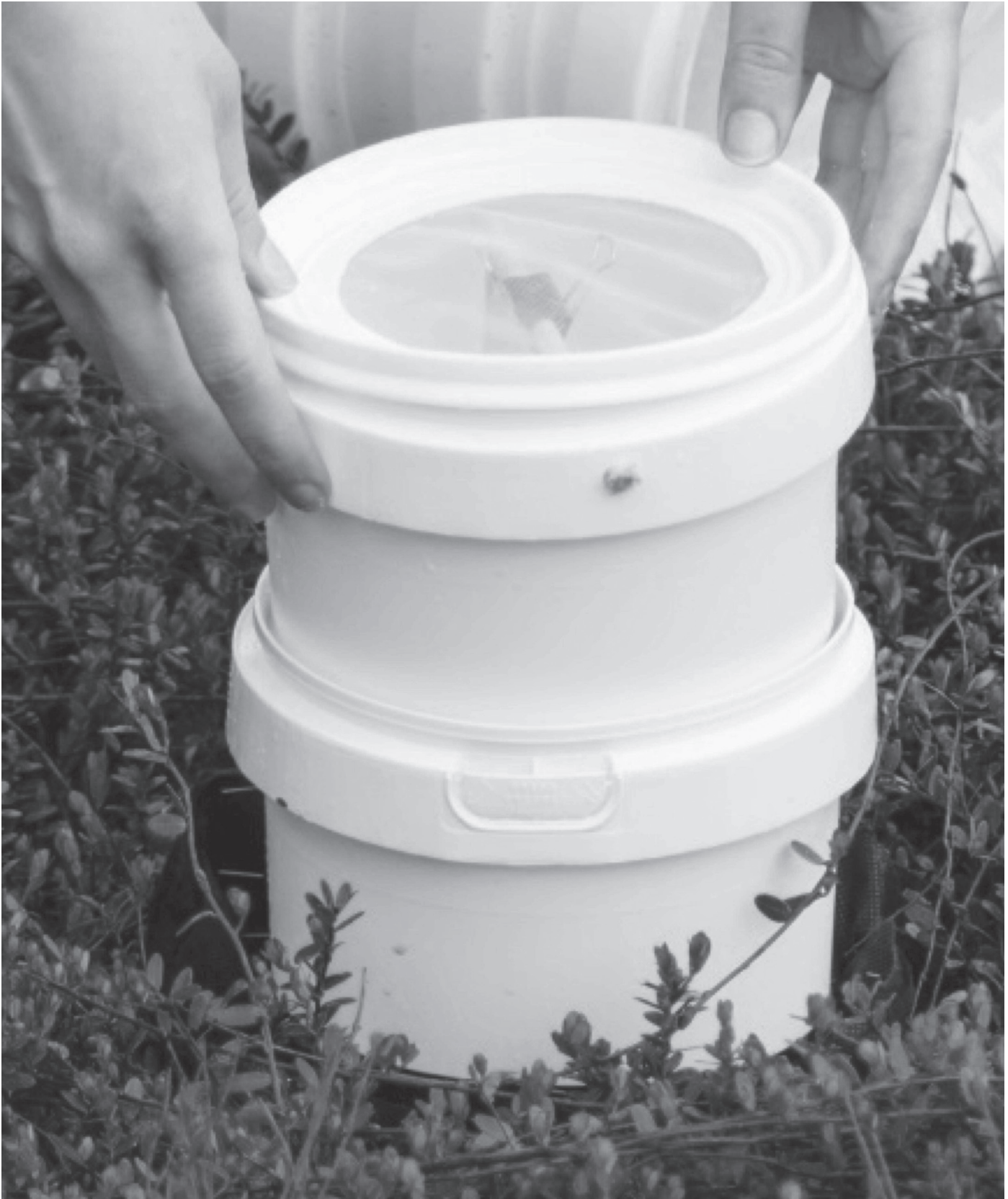
Fig. 1. Bucket-type emergence trap seated into cranberry field. Inner bucket with mesh lid is descending into support bucket.
