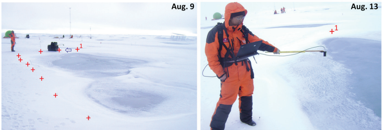
FIGURE 5. Repeated measurements of albedo transects (top) passing through the same melt pond (bottom). The interval between red crosses is 100 cm. the first location on snow is marked in both photos, with last two locations also on snow (MP S/I means a mixture of melt pond snow and ice; water means melt pond water).
