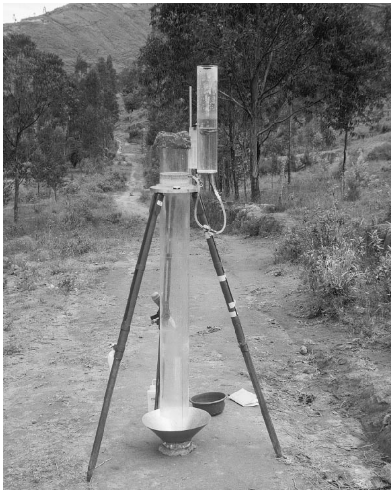
FIGURE 2 Use of a rainfall simulator-infiltrometer on a trail near Quito, Ecuador. (Photo by author)
