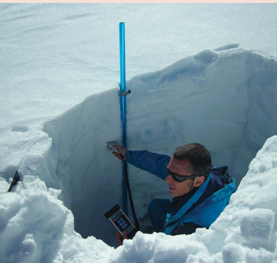
FIGURE 4 PROFILE radioactivity measurement with a Geiger counter and an external probe. (Photo courtesy of Tiziana Corso)
