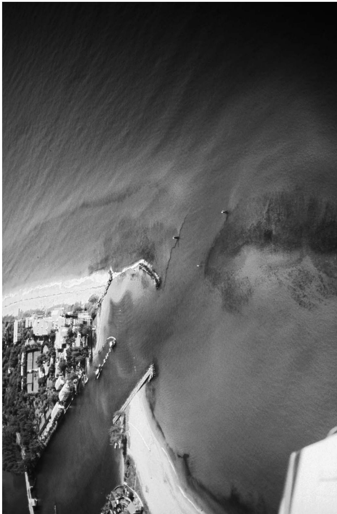
Hillsboro Inlet, Southeast Florida Atlantic Coast. This is one of the few natural inlets in southeast Florida, being an outlet for the Hillsboro River. The inlet was dredged to accommodate deeper draft vessels and is maintained by dredging from the sand trap on the north (updrift) side of the entrance shoreward of the weir jetty designed by Per Bruun, who took advantage of the bedrock outcrop of the Anastasia Formation. Sand is pumped by the floating dredge to the south (downdrift) side of the inlet to help maintain beach width and support littoral transport. This inlet was the first inlet in Florida to bypass 100% of the littoral drift by mechanical means. (Photograph by Charlie Finkl, Department of Geosciences, Florida Atlantic University, Boca Raton, FL 33431, USA).
