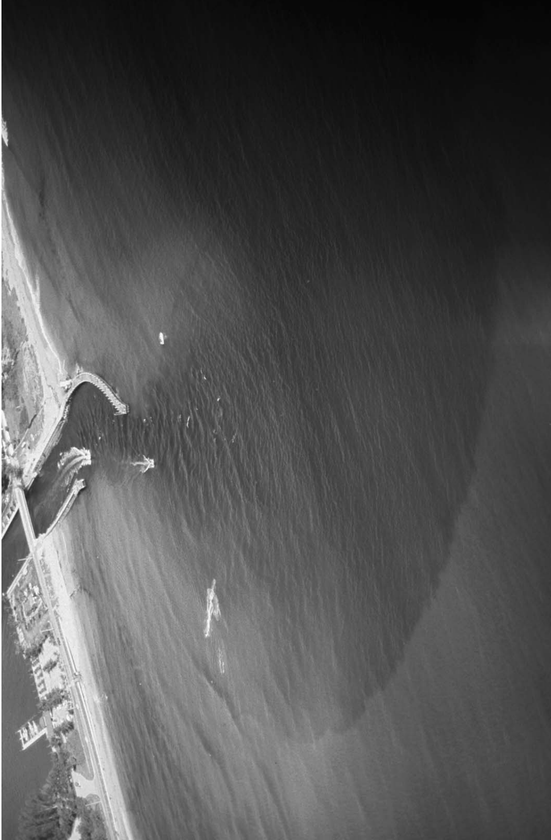
South Lake Worth (Boynton) Inlet on the Southeast Florida Atlantic Coast. This inlet was originally dredged to provide better water circulation in Lake Worth but is now commonly used as a navigational entrance. Water flowing out of Lake Worth in the ebb tide is clearly visible as an oceanic plume in the center foreground as it contains tannic acids that make it darker colored than seawater. Note the curved jetty on the north (updrift) side of the inlet and deflection of suspended sediments in the littoral transport offshore (lighter toned area). The downdrift shore has retreated landward due to littoral drift blocking by the jettied inlet, which causes shore erosion. (Photograph by Charlie Finkl, Department of Geosciences, Florida Atlantic University, Boca Raton, FL 33431, USA).
