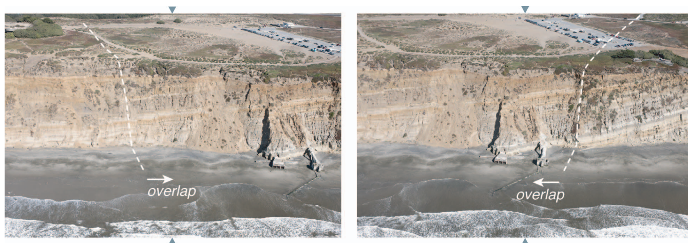
Figure 1. Examples of oblique, aerial photographs of Fort Funston, California, from CCRP (2016). Dashed lines show the approximate overlap between the photos, and photo midpoints are shown with triangles. (Color for this figure is available in the online version of this paper.)
