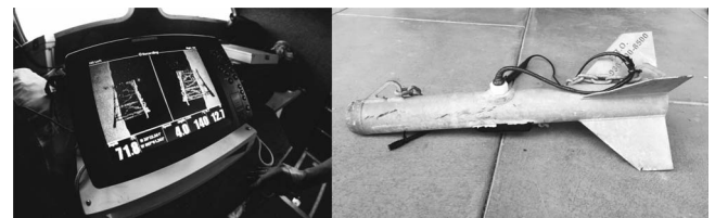
Figure 2. The Humminbird 1198c head unit and towfish with sidescan transducer used in this study.
