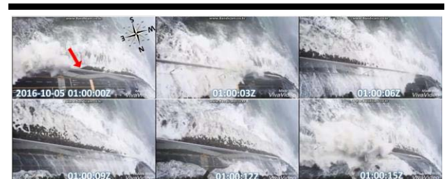
Figure 4. Snapshots of wave trains show the incoming direction, run-up, and resulting overtopping of the dike. Video was recorded at 3-s intervals to determine wave periods.
