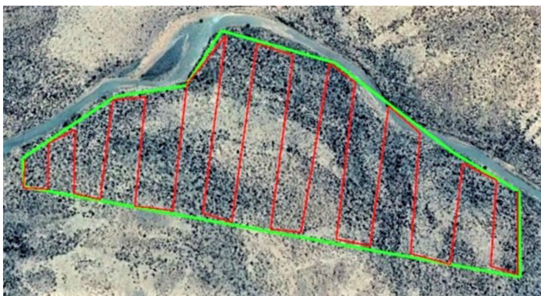
Fig. 3. Example of a field trial search area (green outline) and the proposed survey route (red lines) for the dog-handler team within the search area. Transects were spaced 20 m apart. The direction of movement was decided according to the wind direction upon arrival at the site.
