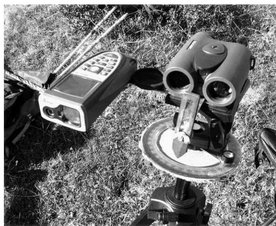
Figure 1. The Animal Locator consisting of the range finder, the tilt sensor and the protractor are combined on the same tripod. A gas bubble level ensures the protractor is horizontal in respect to the ground.
