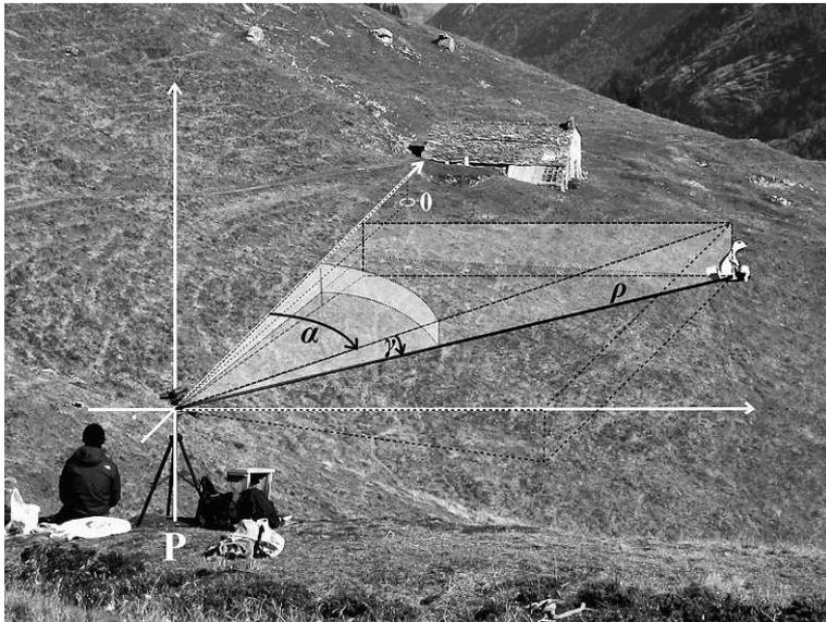
Figure 2. Schematic representation of the angles and the distances needed in order to obtain the position of the observed subject. The instrument is set on observational point  $P_{obs}$ ,  $\alpha_i$  is the orientation of the animal in respect to the zero point,  $\gamma_i$  is the tilt and  $\rho_i$  is the distance from the instrument to the observed subject.
