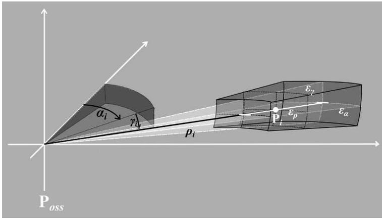
Figure 4. Schematic representation of the errors  $\epsilon_\rho$ ,  $\epsilon_\alpha$  and  $\epsilon_\gamma$ . Errors for each single measure are shown in white (i.e. white line for  $\epsilon_\rho$  and two circular sectors for  $\epsilon_\alpha$  and  $\epsilon_\gamma$ ). Polygon bearing out from the combination of the error parameters is shown with a solid line.
