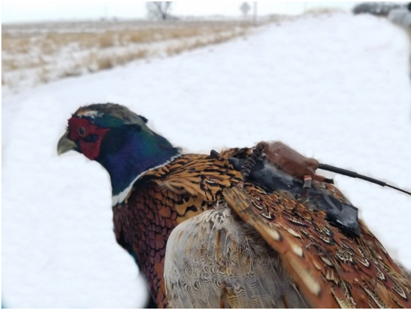
Figure 2. Self-made, low-cost GPS tracker weighing 43 g (<5% of body mass) attached to a male ring-necked pheasant in Beadle County, South Dakota, 2019.
