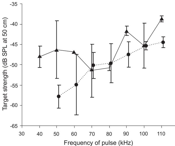
FIG. 2. Mean target strengths at 0.5 m for single frequency pulses reflected from harp traps (circles, dashed line:  $n = 2$ ) and mist nets (triangles, solid line:  $n = 2$ ); error bars show SE of the mean
