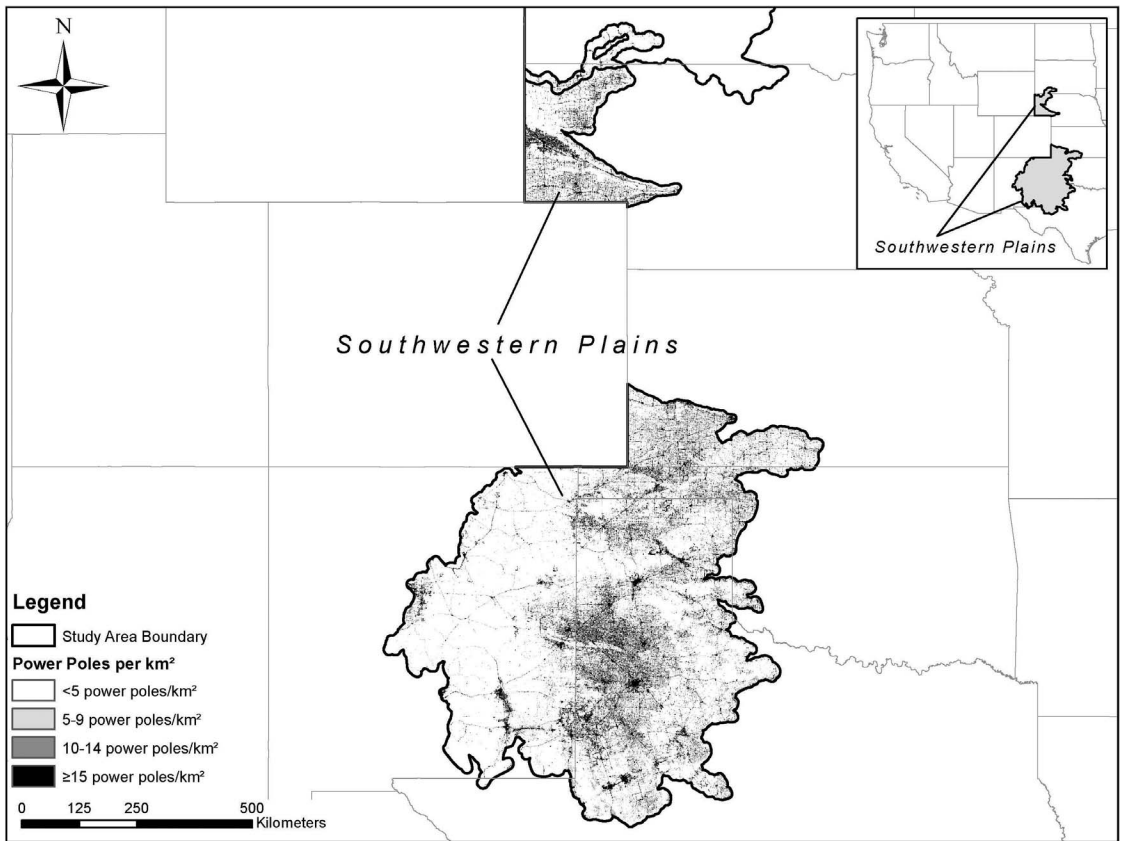
Figure 5. Predicted power pole density from the Colorado and Wyoming model projected to the Southwestern Plains.
