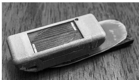
Figure 2. OrniTrack-10 GPS-GSM transmitter with 54-mm long piece of neoprene and flexible plastic cutting board mat extending 20 mm towards the nape. This was intended to cover and divert the bird's nape feathers so they would not obscure the solar panel.
