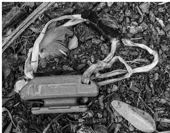
Figure 6. OrniTrack-E10 GPS-GSM transmitter with an intact Y-transmitter Spectra harness, recovered from an adult male Gray Hawk that was apparently killed by a predator. There was no damage to the straps, knots, or the reinforced sternum-connecting-ribbon after the bird wore the harness for 155 d.
