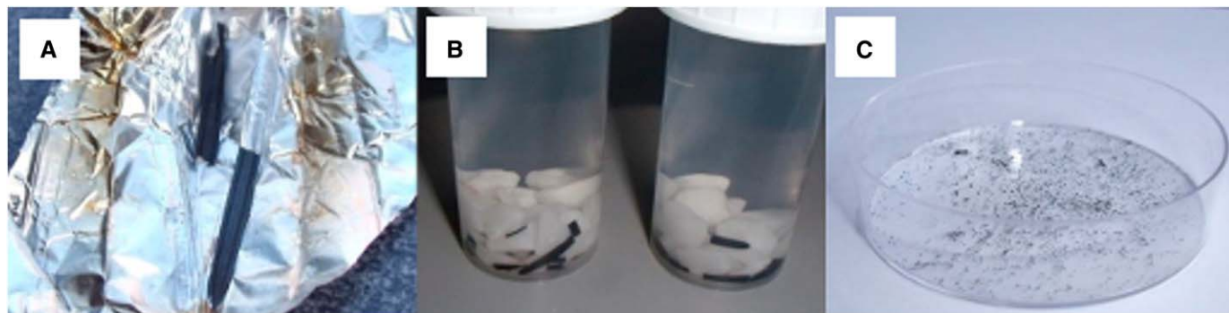
Fig. 1. Charcoal samples, as removed from furnace (A), prior to simulated transport with water and gravel (B), and dispersed on a Petri dish prior to imaging (C).
