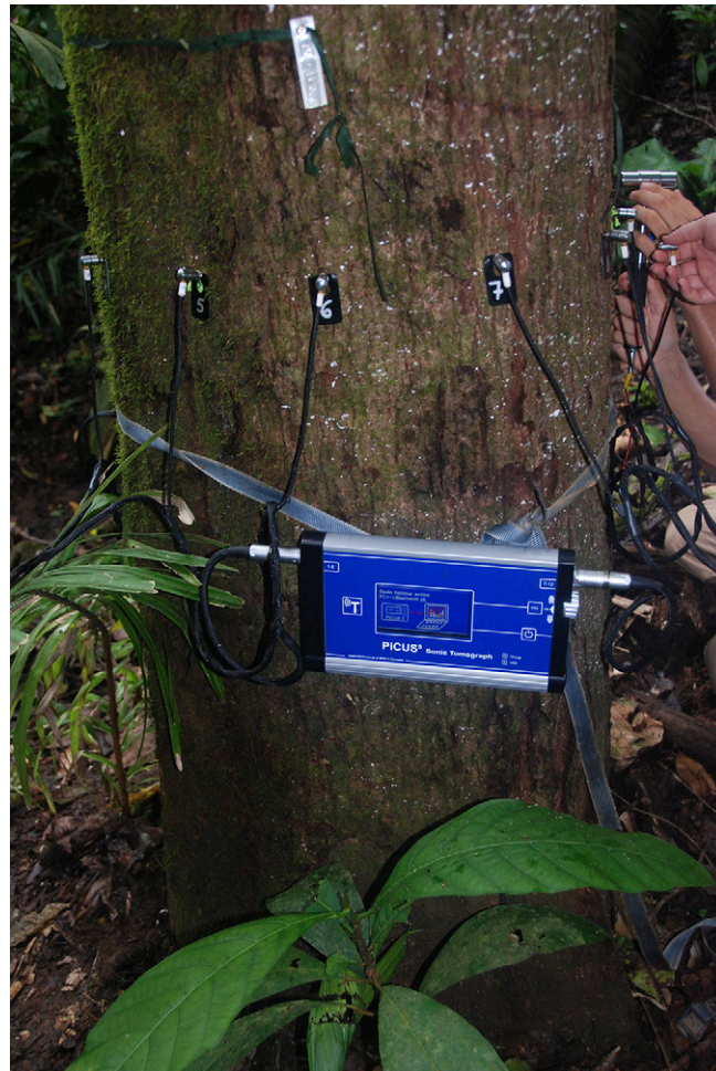
Fig. A1-1. The PiCUS 3 Sonic Tomograph attached to a tree with sensor cables.
