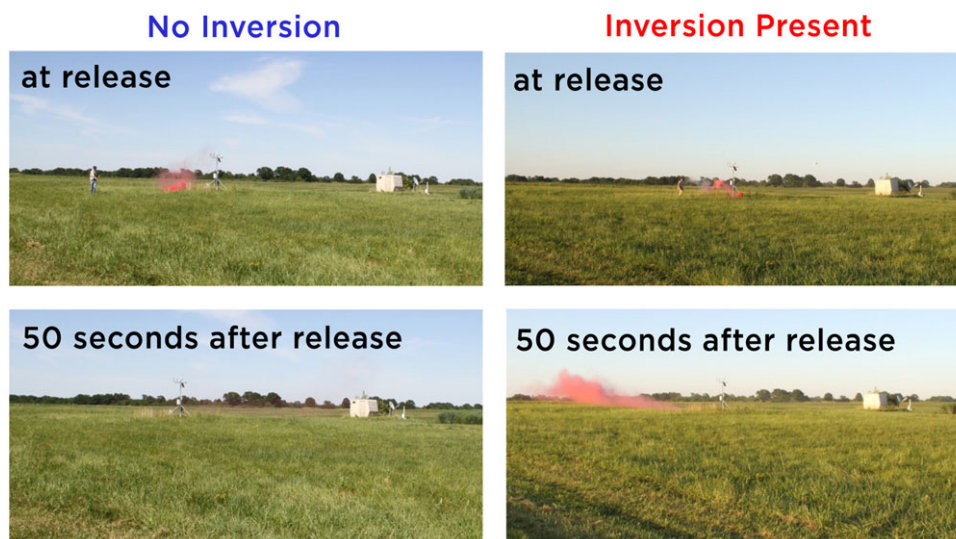
Figure 5. Smoke bombs released at the same site in Columbia, Missouri (2017), during unstable, noninversion conditions (approximately 4:00 P.M.) and inversion conditions (approximately 7:30 P.M.). The smoke plume has dissipated by 50 s following release during noninversion conditions while the plume remained intact during stable conditions.
