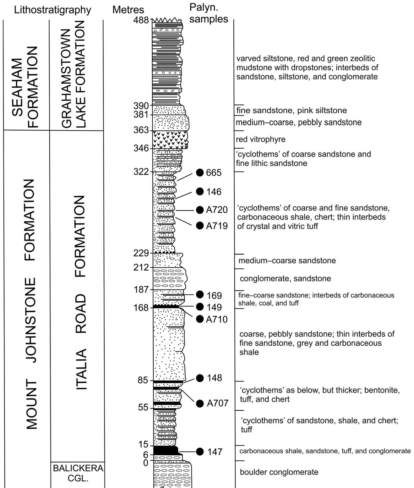
**Figure 2.** Stratigraphic section of the formerly named Italia Road Formation – now included with the underlying Balickera Conglomerate in the Mount Johnstone Formation – as exposed and measured (i.e. before flooding) in the Balickera canal excavation, whence the samples studied herein, as originally by Playford and Helby (1968), were collected. Based on Rattigan (1967a, fig. 4), but see text (section 2) regarding inapt usage of 'cyclothem'.
